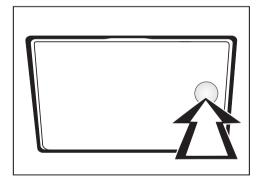
■ Press to open the service panel for the fine filter (see arrow).
